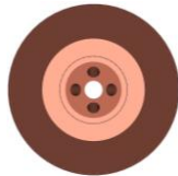
Plasma-nozzle with 4x powder holes (90°)
