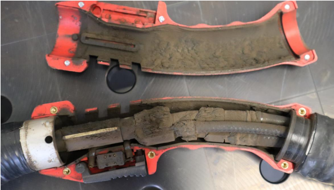
Conventional fume extraction torch
